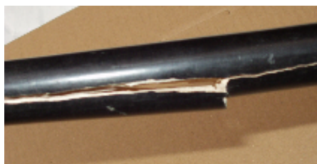
Rupture failures are an indications of straight-grained wood.
